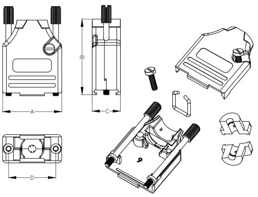
BACKSHELL MATERIAL: PLATING: JACKSCREWS: M3 HOODSCREWS: COMPRESSION INSERT: COMPRESSION SPRING: OPERATING TEMP: DIE-CAST ZINC ALLOY CLEAR CHROMATE FOLLOWED BY BLACK ENAMEL STEEL - BLACK OXIDE FINISH STEEL - BLACK OXIDE FINISH ABS UL RECOGNIZED STEEL, NICKEL PLATED -40°C TO +120°C \* UNLESS OTHERWISE SPECIFIED TOLERANCES ON DECIMAL IS: ANGLE  $\pm 5^{\circ}$ UNIT: MM X.  $\pm 0.38$ X.  $\pm 0.25$
