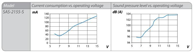
Note : All measurements are made in free air @1 meter @21°C @35% RH. For measurement purposes, the alarm was mounted with mounting bracket "MB1" on a wooden panel.
