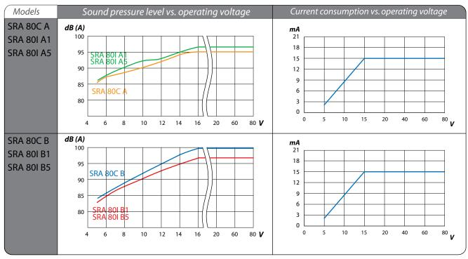
All measurements are made @ 12Vdc @ 1 meter in free air @ 21°C.
