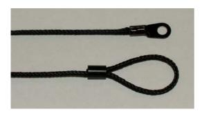
**2.** Depending on the version crimp lanyard with crimp barrel or ferrule with tool.
