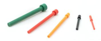
Sealing plugs are used to seal unwired contact cavities. After installing unwired contacts into unused cavities, insert knob end of sealing plug into grommet until it bottoms against the unwired contact per illustration. Install sealing plugs with standard contact insertion / extraction tools.
