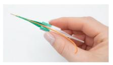
• When inserting the contacts, start with the central cavities.
