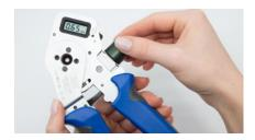
Positioner for 080.000.072.000.000: Insert the positioner into the crimping tool. To do this, turn the tool around so that the rear side is facing you. Insert the positioner with bayonet pin into the adapter ring and turn 90°. The positioner locks into place.
