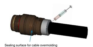
6. Fasten the shield braid to the backshell by means of crimping or by using a metal band. More information see page 4. Encapsulate the interior of the backshell to secure the soldered points (ODU advise WEVO-2K-casting resin PU552FL)
